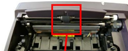
Clean interior of Printer using air
