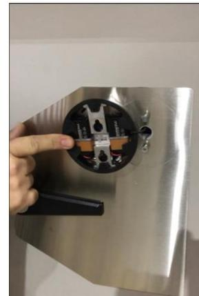
Turn keypad around to access and change batteries.
